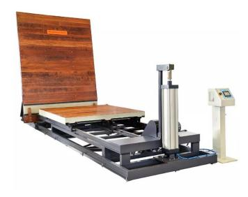
This machine is designed to determine the resistance of furniture to impact. A motor-drive chain is used to control the movement of the workbench, on which the furniture hits the stop plate at a given speed. After testing, check the furniture for damage.
